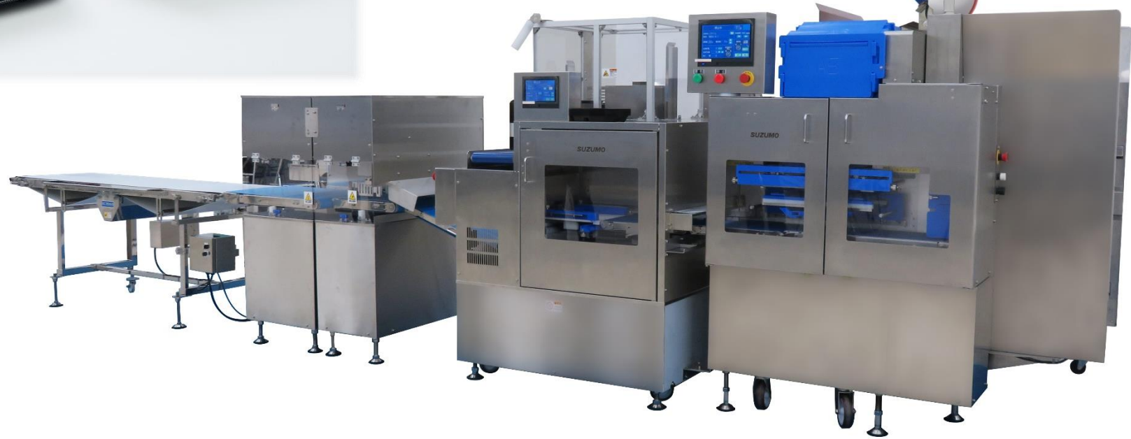
Filler line: Multi-filler with scale / Multi-former / Container filler with final scale
