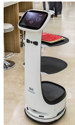
New generation serving robot that realizes 50cm aisle width travel
